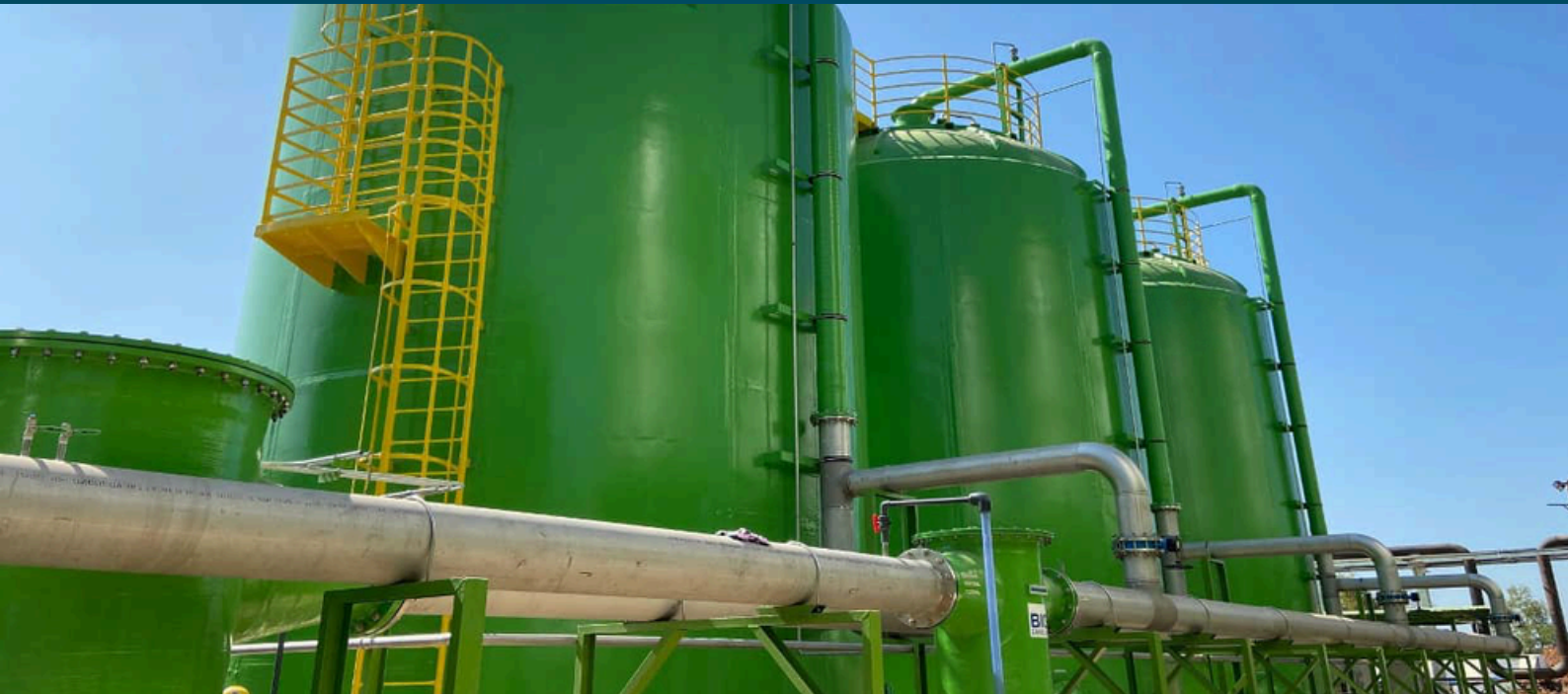
Plant: KSL Green Innovation PCL Thailand. Capacity 5,000 M3/h (2,941 scfm) biogas 15,000 ppm H 2 S
